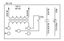
**Note:** Record the lead wire color with it's corresponding terminal for future reference. Unused transformer input leads must be insulated.
