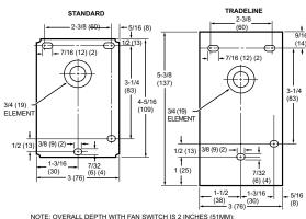
NOTE: OVERALL DEPTH WITH FAN SWITCH IS 2 INCHES (51MM); MODELS LESS FAN SWITCH ARE 1-5/8 INCHES (41MM).
