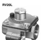
VENT LIMITING DEVICE When using the vent limiting device, the regulator must be mounted in a horizontal upright position.
